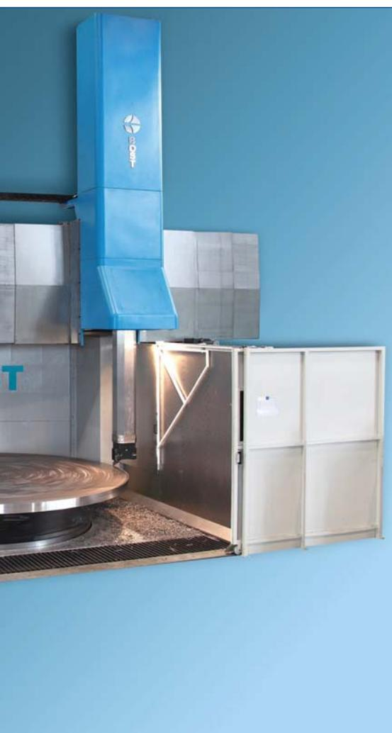
*The new CNC vertical turning and boring mill makes it possible to work large lathe parts with a diameter up to 4000 millimetres and lathe height of up to 1800 millimetres.*
