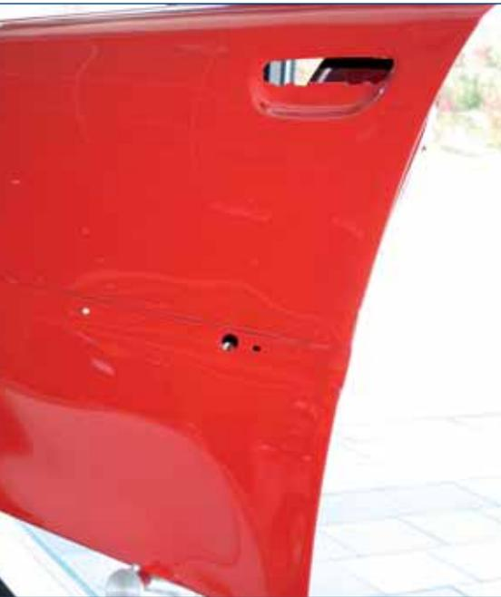
*This demonstrator of an enamelled car door made from magnesium was made in the TeMaK growth centre.*
