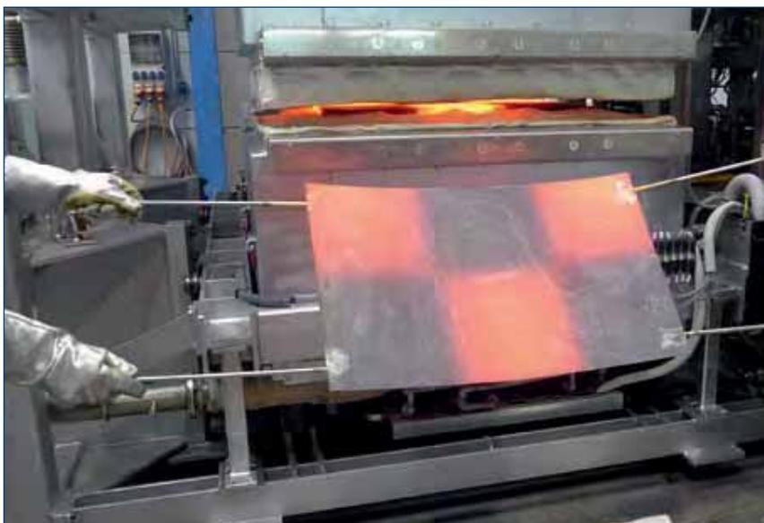
**An intelligent press hardening line has been placed in operation at the Fraunhofer Institute for Machine Tools and Forming Technology IWU. The institute's internally developed process chain promises to accomplish the Industry 4.0 idea of controlled press hardening of near-series components. The core feature is a networked process management system across the entire process chain.**
