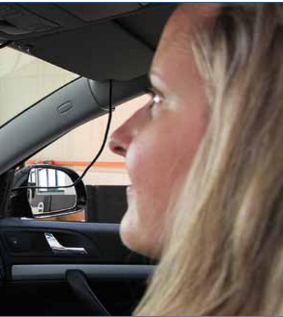
Multisensor monitoring of the vehicle interior. Among other things, this records driver well-being. This information makes it possible to optimize the transfer of control and driving style during automated driving.
