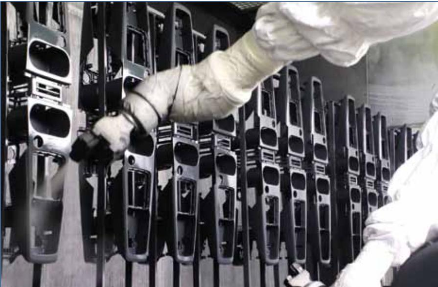
Photo p. 24: Interior parts being prepared for electroplating at SAXONIA Galvanik.
