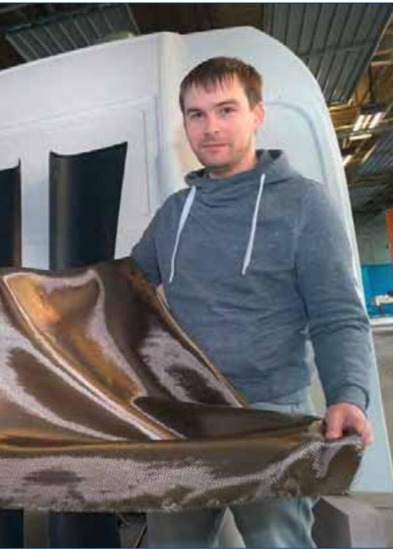
Alpha Sigma founders Michael Jakob (left) und Fabian Liesch, with the material used to make basalt-fiber composites, such as automotive engineering prototypes and small series.
